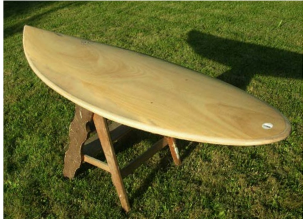
Surfboard using sandwich technology (Koto veneers).
